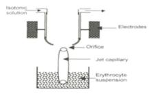
Figure 6: Electro encapsulation technique
