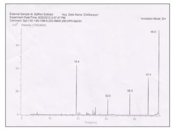
Figure 4. Gas chromatogram of the etheral extract of saffron stigma
